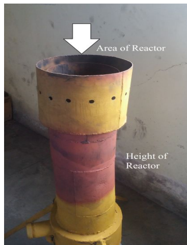
Fig .3. Cross-Sectional Area and Height of the Reactor.
